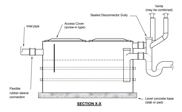
**NOTE:** Baffle and internal pipe configurations vary according to tank type capacity and/or customer requirements. All attempts should be made to ensure external connections correspond as close as possible to these drawings.
